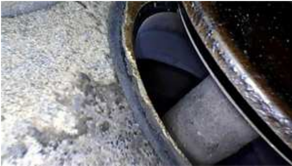
Closeup of the healthy O-320 exhaust valve, with a good view of the seat and valve-sealing surface.
