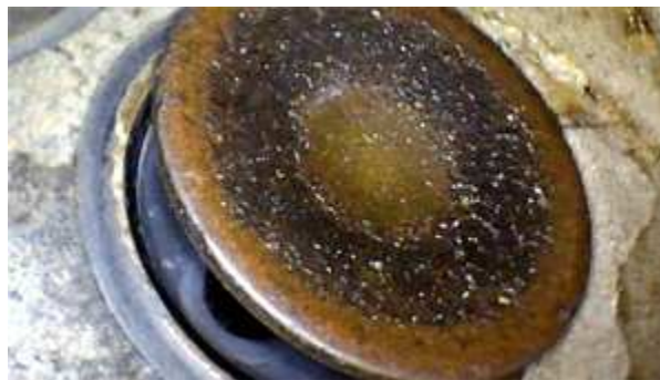
Lycoming O-320 exhaust valve. Note the symmetrical "bullseye" appearance indicating a healthy valve.
