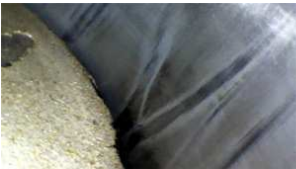
O-320 cylinder barrel and piston. This jug is very worn: Note the vertical scoring and lack of crosshatch.
