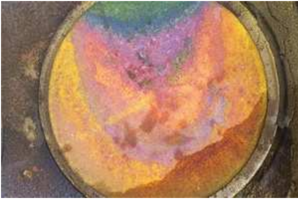
This is a very sick exhaust valve on the verge of failing catastrophically. Note the asymmetrical appearance: That's bad!
