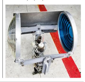
The halogen bulb is positioned in the center and rotates with the clear and colored lenses, while radiating a total of about 15,000 lumens of light energy. At 20% conversion efficiency, halogen bulbs are about twice as efficient converting electrical energy to light as incandescent bulbs, but they still waste 80% of the input, and also run at higher operating temperatures than incandescent bulbs, making cooling a constant concern:
