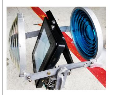
One panel shines through the clear lens, and one through the green lens (which looks blue in the picture due to the wonders of cell phone photography). By FAA specs, the lenses are angled upward at six degrees, and the light panels another six degrees beyond that to fill the Fresnel pattern.
