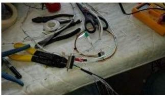
The instrument panel was a formed, blank piece of aluminum. After using patterns of instruments for the layout, the panel was cut with a water jet. This was a huge time saver over drilling and punching holes with Greeley punches, and the result was excellent. Preliminary wiring was done and harnesses were made for the avionics.
