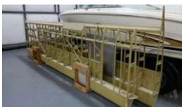
The wings were partially assembled from the kit builder. There is a long story here, but suffice it to say they were not in the stage that usually leaves the kit builder. I needed to install the flap and aileron hangers, make the tank covers, install the trailing edge pieces (false spar) and all pulleys and brackets.
