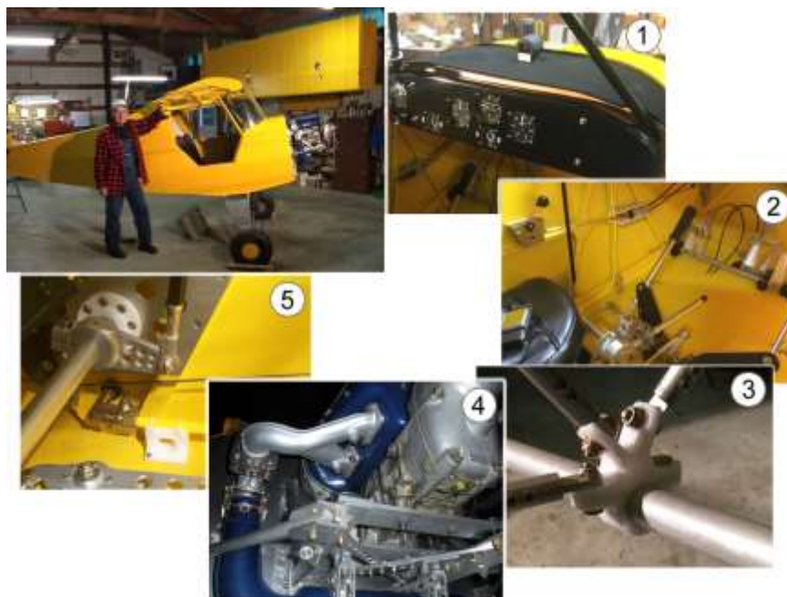
Plane and builder with CAD-designed and machined parts: 1. Fiberglass molded panel.
