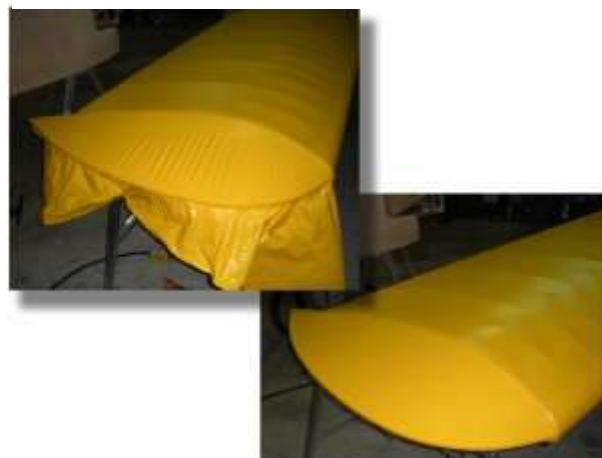
Wingtip before and after heat-shrinking.
