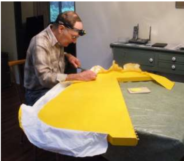
Oratex process is clean and odor-free; small parts could be done inside on the kitchen table.
