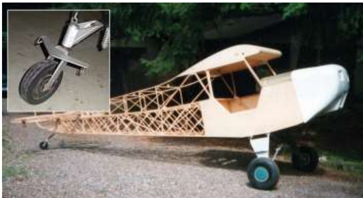
Main wheels are Piper; tailwheel fork & bearing head are from a friend's wheelchair.
