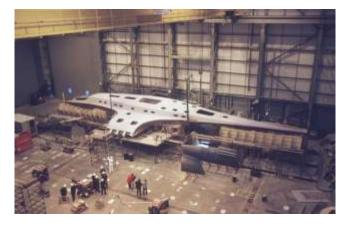
The *Cable & Wireless Adventurer* was designed and built to circumnavigate the globe in less than 80 days, to break the world record held by the US. Equipped with mostly British-designed, state-of-the-art navigation and communications equipment, the unique 115-foot stabilized monohull, twin-diesel powered vessel, left Gibraltar on 19 April 1998 on its pioneering 26,000-mile world-wide journey.
