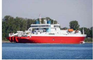
Kevin is the Captain of the CABLE INNOVATOR, a deep-sea vessel designed to lay underwater cables for telecommunications, electric power transmission, military, or other purposes. These cables are the undersea internet network cables providing our connections to distant places. It was built in 1995, is currently sailing under the flag of UK and is berthed in the Port Angeles Harbor. Its mission is cable repair on the west coast from Alaska to Mexico.
