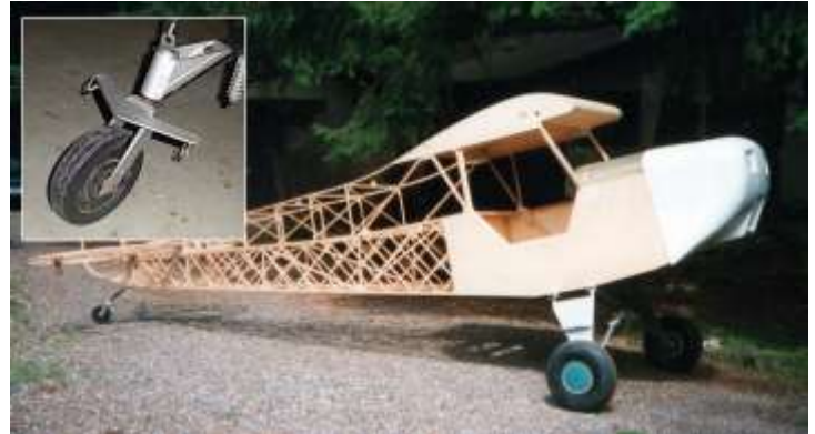
Main wheels are Piper; tailwheel fork & bearing head are from a friend's wheelchair.
