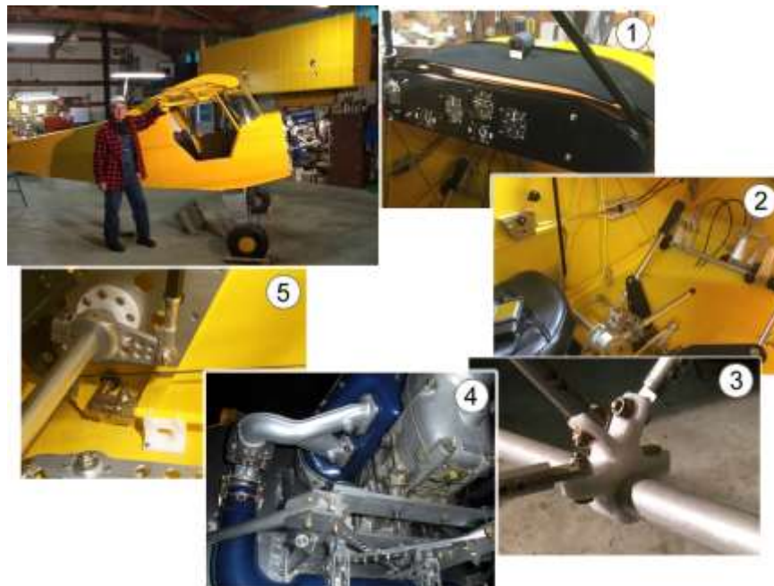
Plane and builder with CAD-designed and machined parts: 1. Fiberglass molded panel. 2. Cockpit layout w/dual controls. 3. Jury strut connector and strut end. 4. Engine mounting. 5. Flap crank and support bearing.
