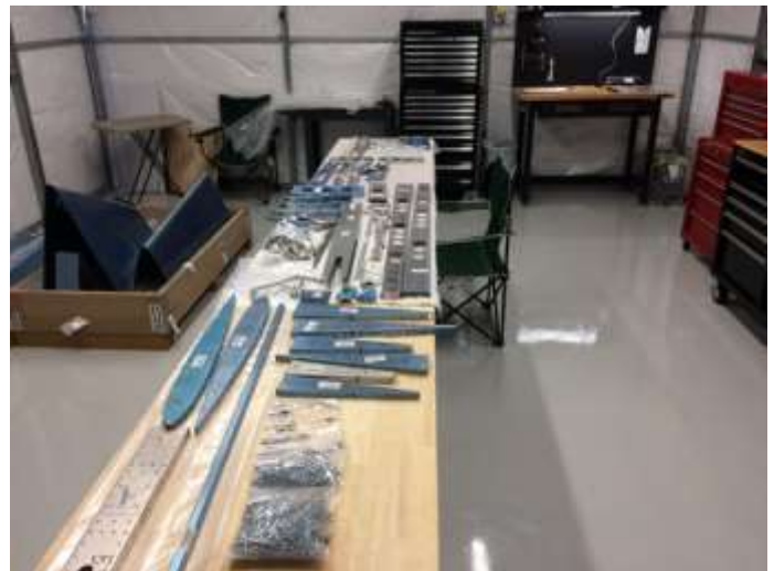
Empennage Kit – Inventory and Inspection
